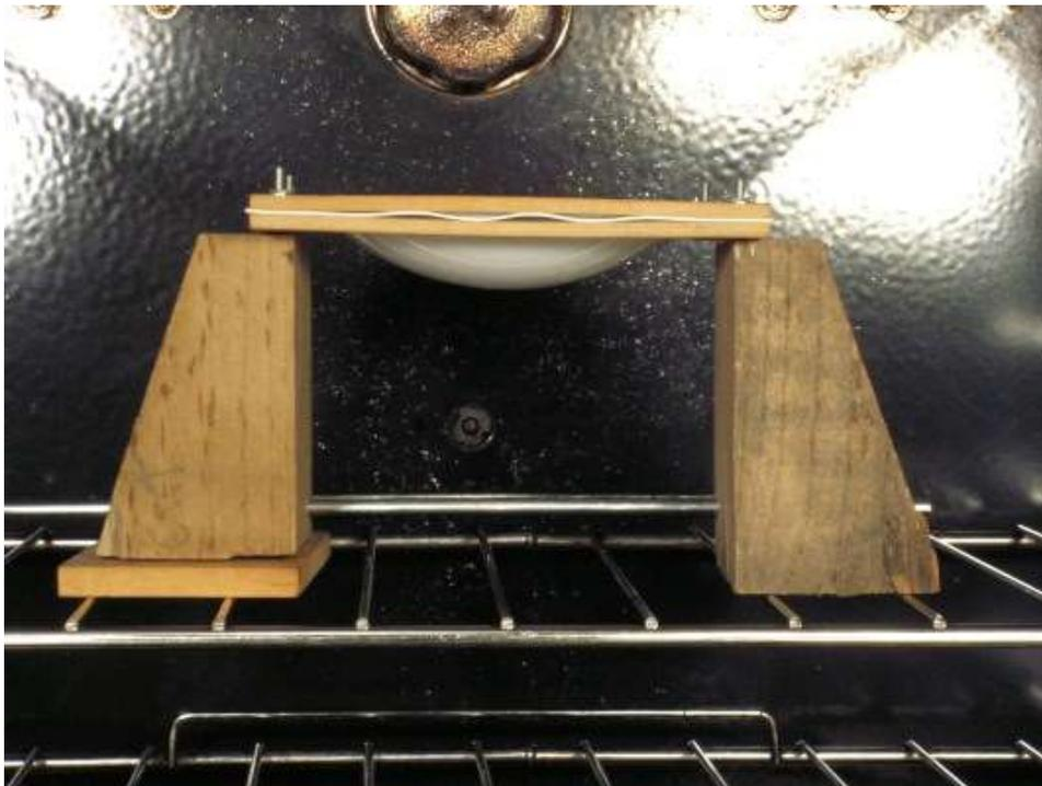
5. Quickly (but carefully, the frames do get warm, I use padded gloves) remove the frame from the oven and centred over the *Master Pattern* place down on the *Vacuum Box*
