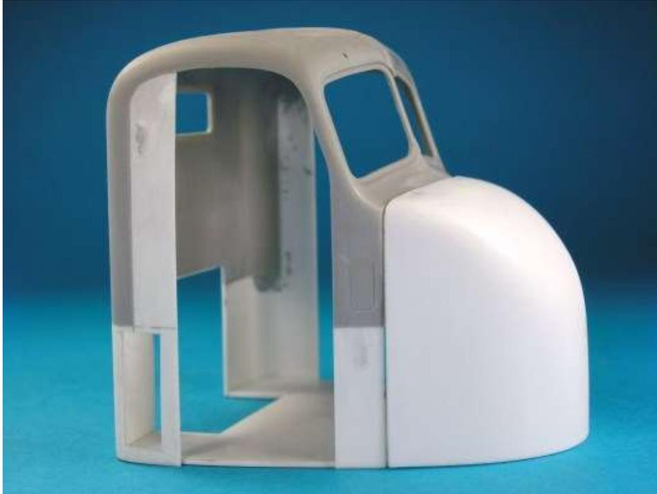
11. If the plastic did not pull down completely over the *Master* you can sometimes place the same sheet frame back in the oven and reheat it and try again. Otherwise its try again with a fresh sheet and try leave it heating a little longer.
