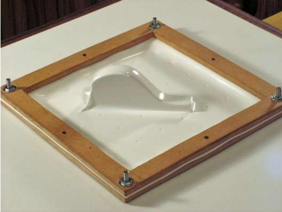
7. Remove the raising blocks from the oven and switch off the oven
